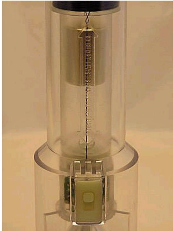
The see-through shaft of the NightStar reveals an inner chamber, within which the one inch long magnet moves back and forth. In the center of the shaft, a tightly wound spool of blue colored wire rests, ready to react to the energy generated by the repeated passing of the magnet. The two ends of the
