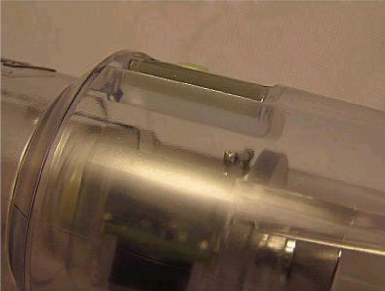
Instead, there is a small metallic plate on the underside of the switch. A couple millimeters underneath that plate is a raised metal bar. When the switch is in the forward position, the small metal plate is passed directly over the metal bar, which reacts to complete the circuit and turn on the light. Sliding the switch back will then break the circuit and turn off the light. Clever!
